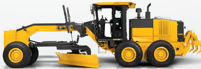
JOHN DEERE 772G motor L6 9.0L 9000CC 549CID (Turbo 6090H PowerTech Diesel)
